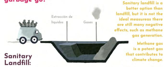
It is a planned disposal of waste. For example, the bottom of the landfill is sealed to prevent contamination of the subsoil, and the garbage is compacted with heavy machinery so that it takes up less space.
